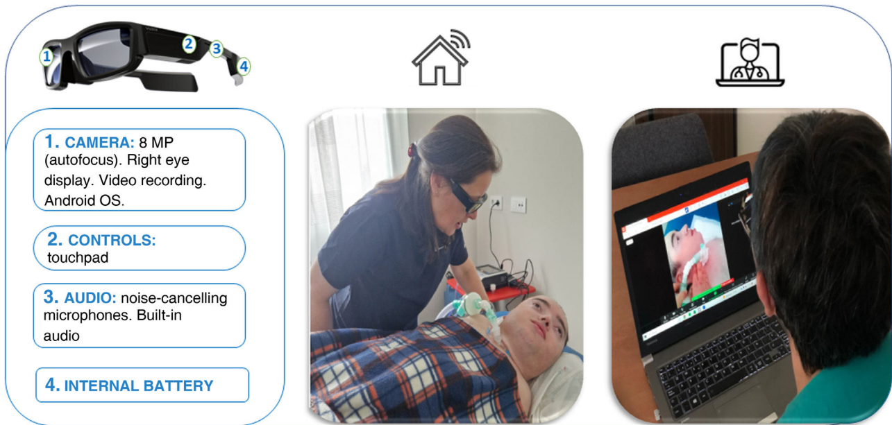
Figure 1 Pictures of the virtual appointment and characteristics of the Vuzix Blade Upgraded smart glasses.
